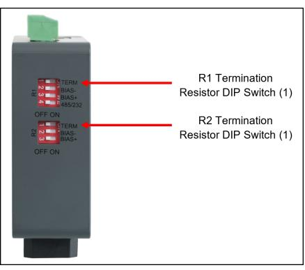
If the gateway is the last device on the serial trunk, then the End-Of-Line Termination Switch needs to be enabled. **To** enable the termination resistor, move the TERM dip switch to the right in the orientation shown in above.
