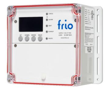
The Frio S1-A is a fully featured single-circuit heat trace controller with integrated Ground Fault Equipment Protection (GFEP). The Frio S1-A can be used for a variety of applications including freeze protection, process temperature maintenance, hot water maintenance (HWM), snow melting, roof & gutter protection, and grease waste lines.
